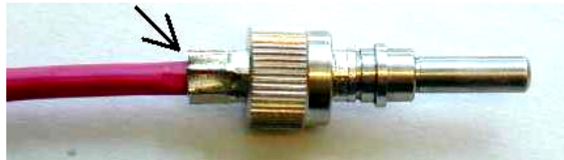
Figure 5. SMA termination with boot removed. Arrow indicates possible water entry point.
