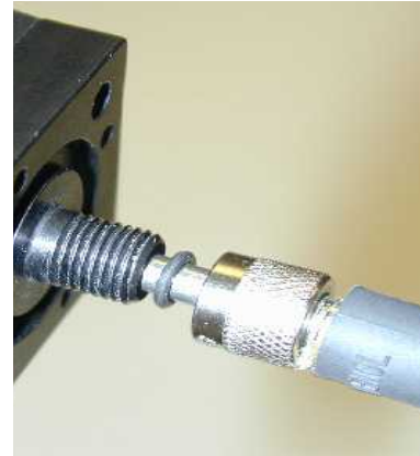
Figure 3. Inserting SMA connector with o-ring in place
